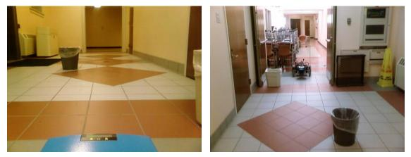
The vehicle was able to move in the hall without hitting the obstacles. Overall we were satisfied with this design aspect. If given more time, a more robust code could be written. Now, with the current code, there is oscillation in the system because there is a delay from when the laser scans to when it sends a command to the motors, to when it takes another scan.
